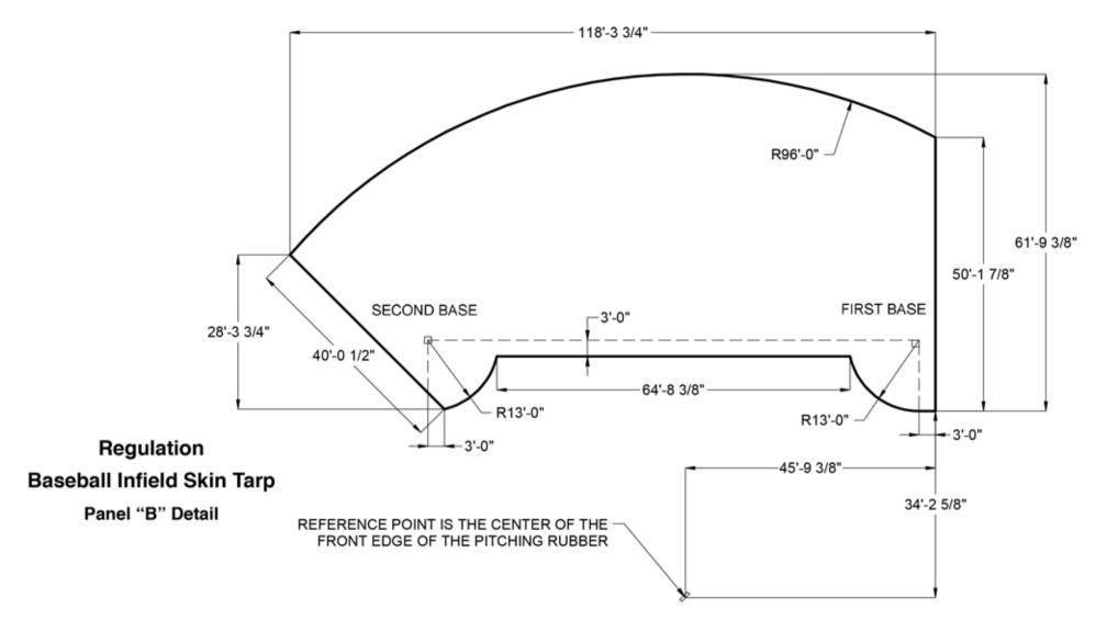
DIMENSIONS SHOWN ARE TO 1/8" PRECISION. ACTUAL PRODUCTION TOLERANCE IS +/- 3 TO 4 INCHES.
